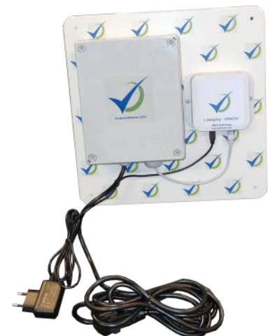
XB040 - 4G router (+ WIN-Gateway on a mounting plate)
